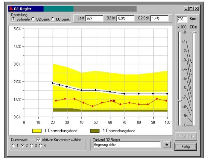
Figure 3: Visualisation of the O<sub>2</sub> /CO setpoint-curve with its monitoring-band-gaps when using the ETAMATIC's OEM integrated O<sub>2</sub> /CO control
