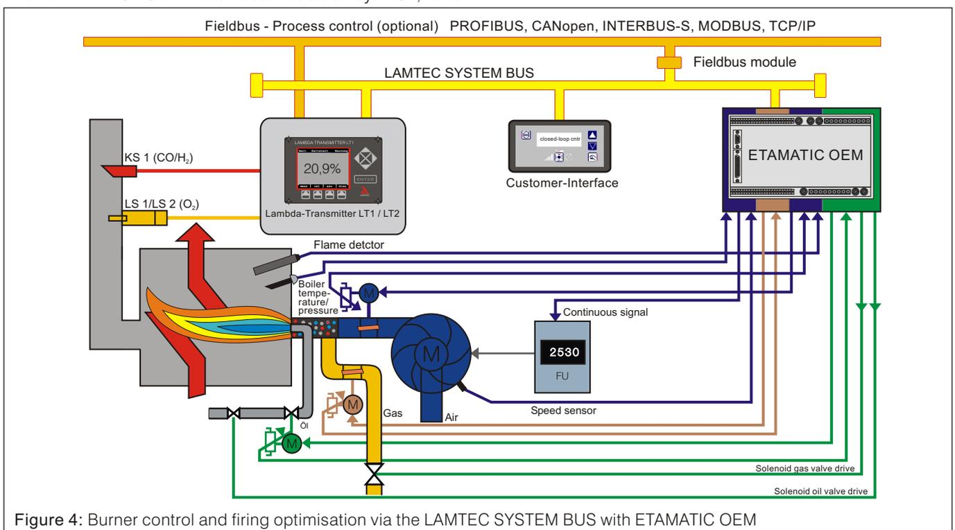
Figure 4: Burner control and firing optimisation via the LAMTEC SYSTEM BUS with ETAMATIC OEM
