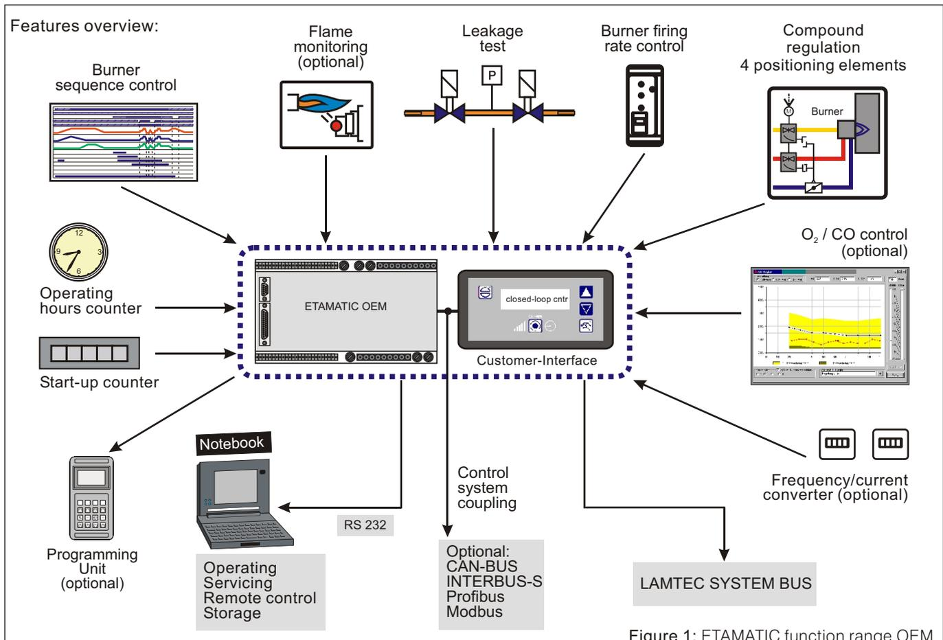
Figure 1: ETAMATIC function range OEM
